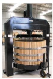
1300 litre in ground model with wheeled trolleys
